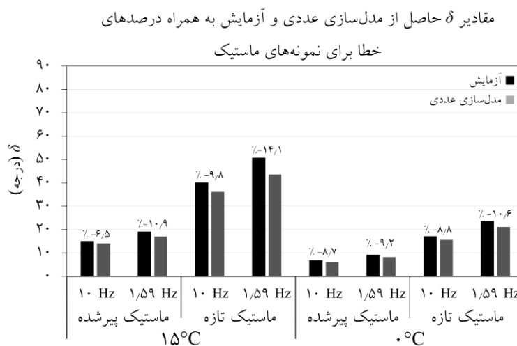
Fig. 22. \delta values obtained from numerical modeling and experimental testing, along with the percentage errors, for the mastic samples
